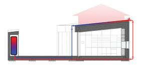
Thanks to this system, the heat pump performs only reduced cooling functions, because it has to work in cooling mode only under high ambient temperatures (~ 35°C). This saves a significant amount of energy on the cooling side. If the water did not cool back sufficiently at night, the heat pump would help out for cooling during the night. Naturally, rain water will be filling up the tank.
