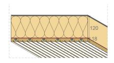
It is the individually developed dropped ceiling that we use primarily for cooling through the integrated piping system. Thanks to the thin MDF board and the thermal conductive paste slushed into the grooves, its heat transfer is 50 W/m². Above the piping there is thick thermal insulating layer.
