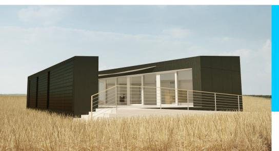
The integration of solar panels are not just an aesthetical issue. The PV modules are mounted as a complete façade and roof cladding elements, substituting the normal covering of the house's surfaces.
